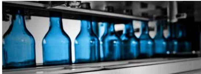
generation. Furthermore it is not only equipped with high-performance cameras but also with unique X-ray strobes. They generate very clear pictures of the complete bottle base using a minimum amount of radiation. These are combined and evaluated by the HEUFT *reflexx<sup>2</sup>* image processing system in real time. Even such faults are made visible which were not detectable in the past. Thus the self-explanatory device makes a highly precise empty bottle inspection simply easy.
