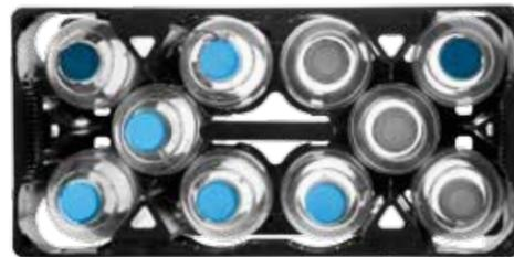
They cause obstructions in the unpacker if they are out of shape, defective, dirty or the incorrect brand. The efficiency and productivity of complete filling lines are also affected if they contain too many non-brand bottles: therefore it is necessary that returned returnable bottle crates with such faults are detected and sorted out in good time – with the HEUFT *LGX*! It examines their dimensions and complete insides optically
