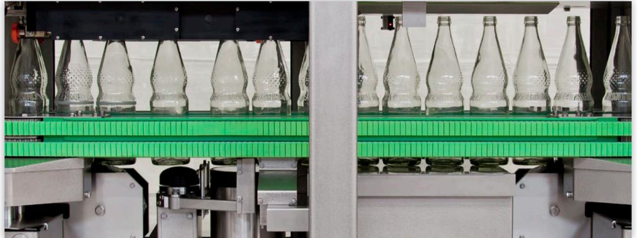
Servo-controlled conveyor belts align the bottles exactly.
