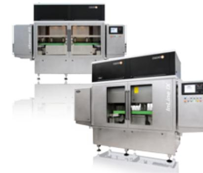
The unprecedented detection reliability of the HEUFT *InLine IX* empty bottle inspector is due to the in-house developed X-ray technology which has only been used in the full container inspectors of the HEUFT *eXaminer* series until now. In contrast to conventional X-ray scanners radiation is only emitted precisely at the moment when a bottle to be examined is in the inspection area and that in the form of an X-ray flash which only lasts a
