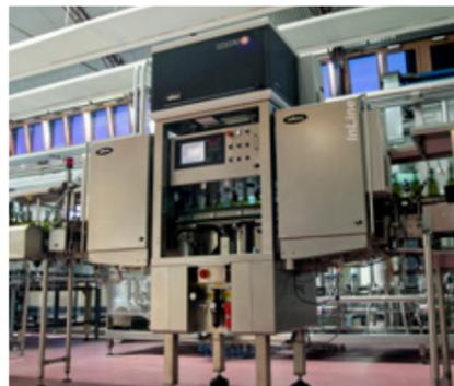
The additionally integrable sidewall inspection carries out a continuous inspection of the empty bottles.
