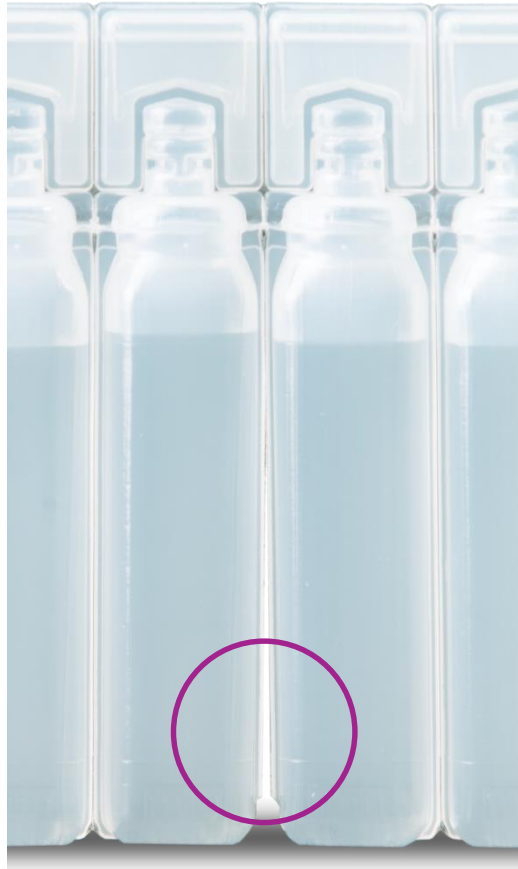
Forming defects interrupted connector
