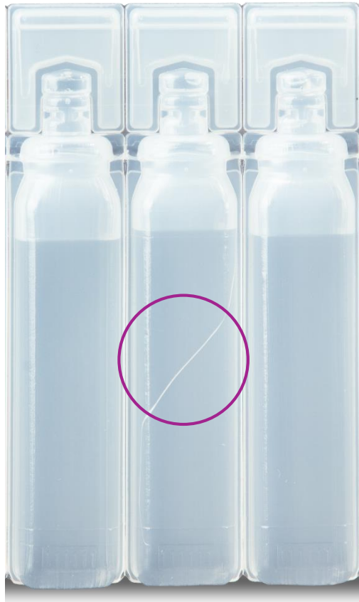
Body damage scratch
